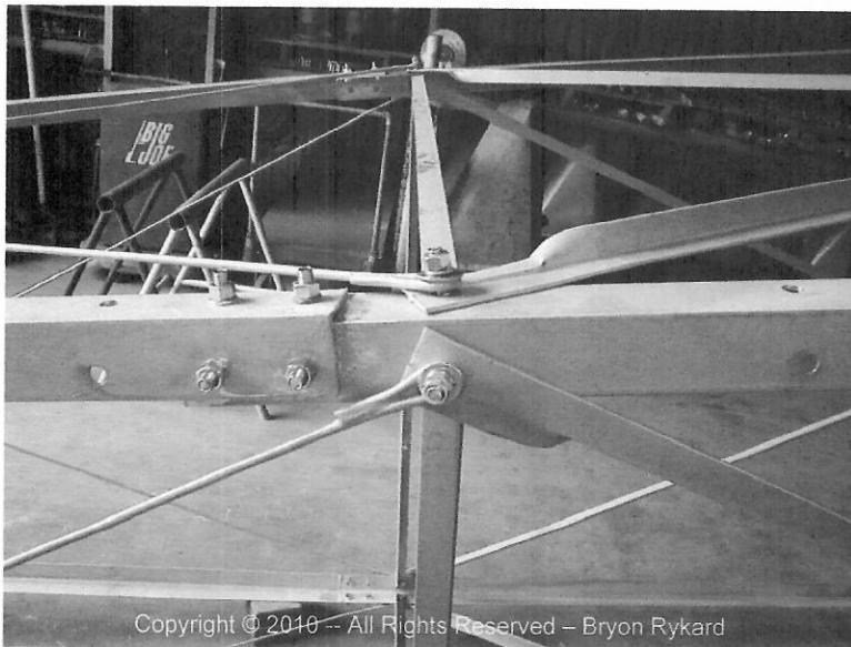
Copyright © 2010 -- All Rights Reserved – Bryon Rykard Figure 12: Begin tightening the nuts at this point of the tower.
