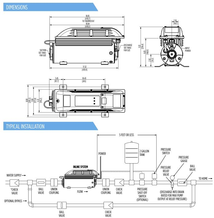
NOTE: These optional components are shown in a typical installation diagram. They should be used at the installer's discretion as required for particular applications. \* When connected to a municipal system, if the plumbing does not have a backflow prevention device, a check valve is required on the incoming water supply line. If installed on a cistern, the check valve should be passive or be eliminated.
