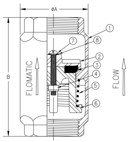
Max Temp 180°F (82°C) Max Pressure 400psi (28bar)
