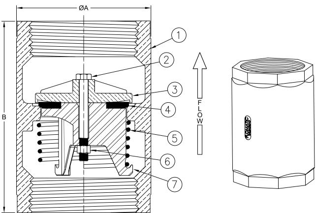
Max Temp 180°F (82°C) Max Pressure 400psi (28bar)
